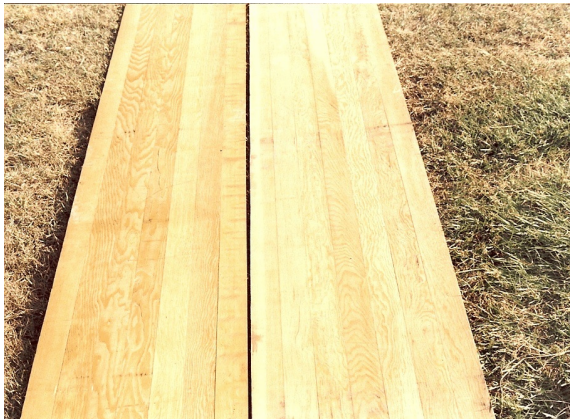
Flame Safe Treated Wood (before test)
