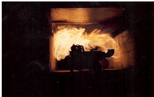
"Fire End" of Steiner Tunnel
